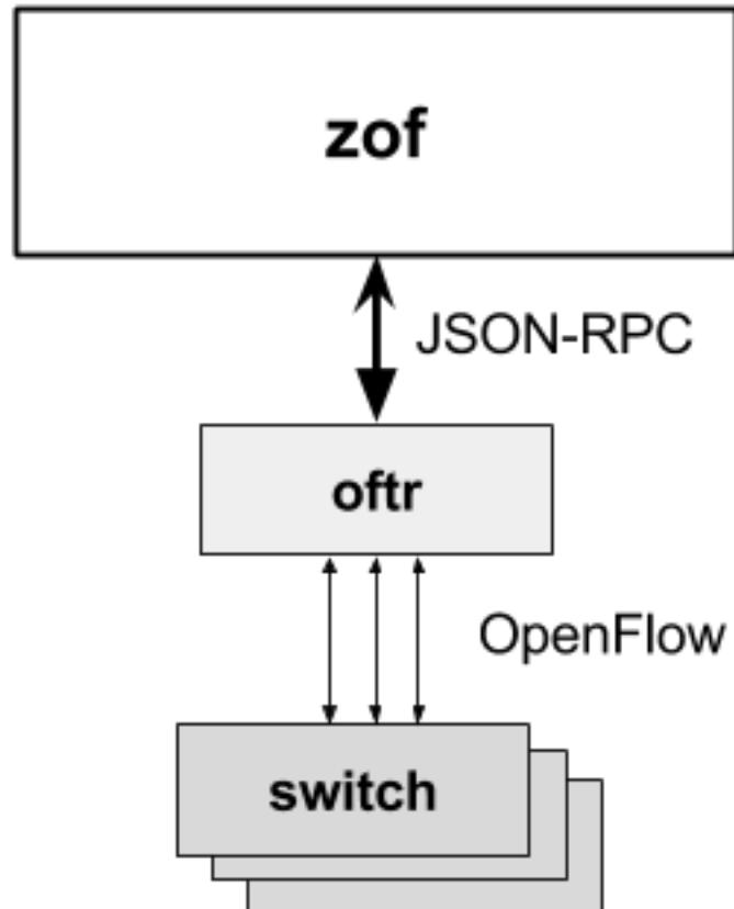
Fig. 1.1: Architecture: The oftr process translates OpenFlow to JSON.
